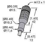
Connector socket M12x1 straight, 5-pin
